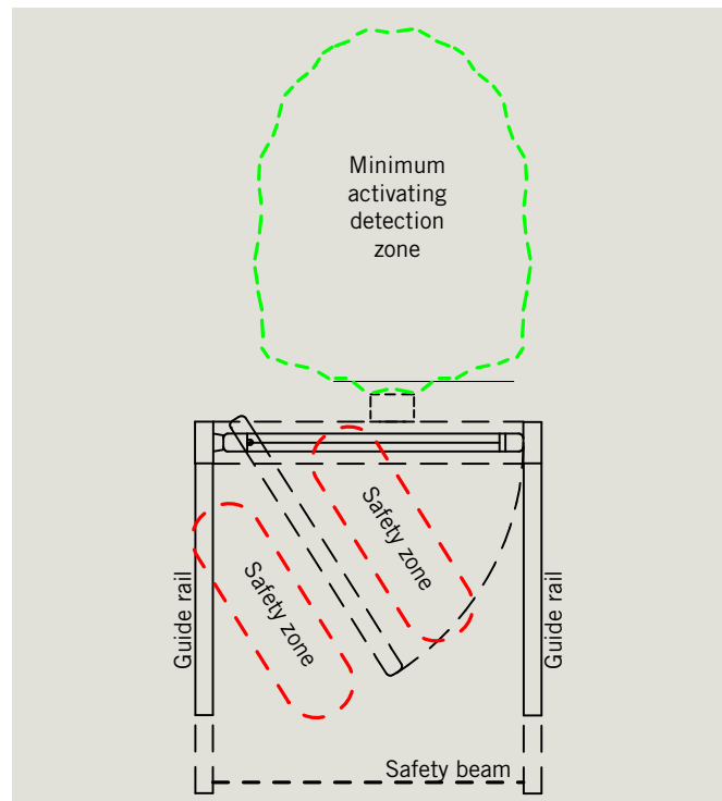
Fig. 5.1.2 One way traffic, door mounted presence sensors
