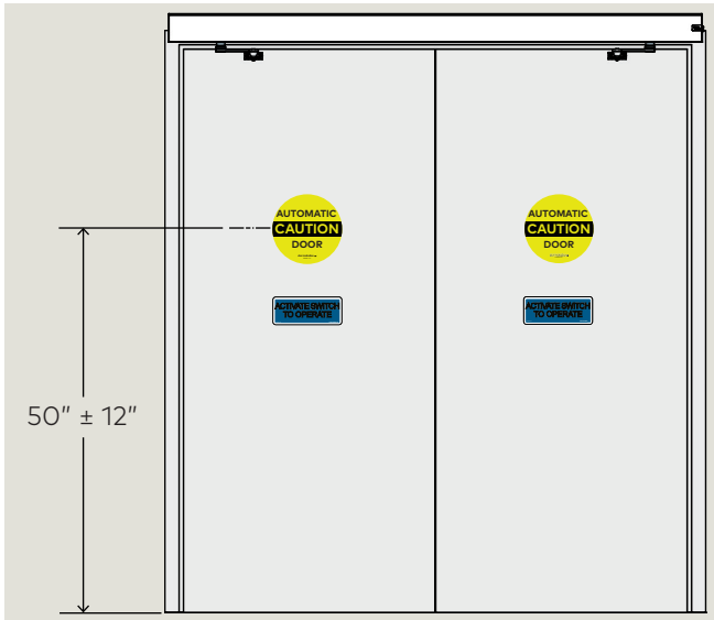
Fig. 7.6.3 Push/Pull, Push to operate
