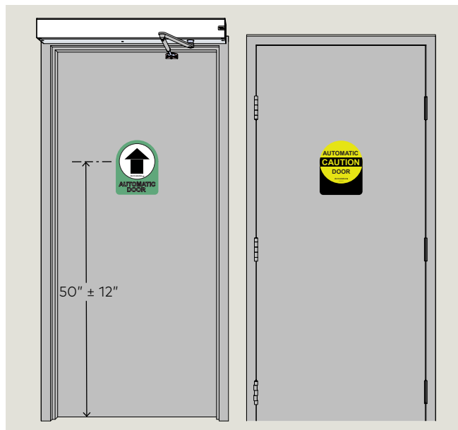
Fig. 7.3.2 One decal, two way traffic Non-swing side Swing side
