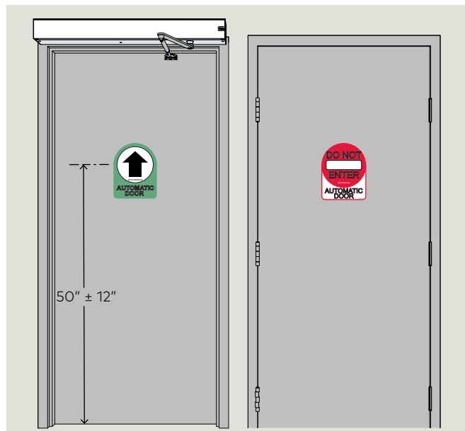
Fig. 7.3.1 One decal, one way traffic Approach
